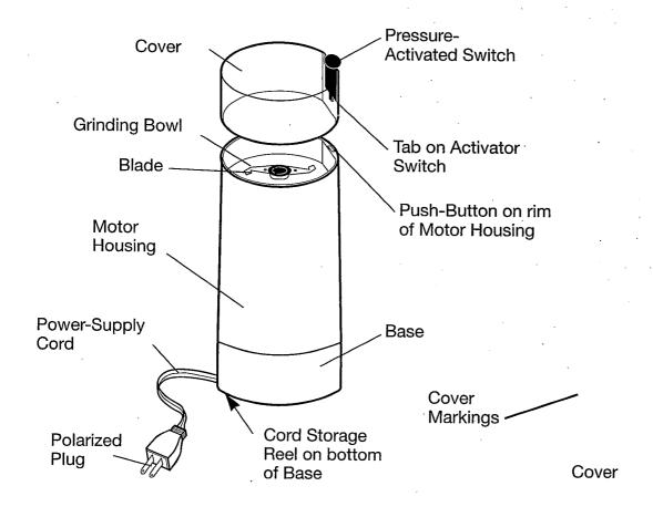
Your Grinder is for HOUSEHOLD USE ONLY. Place it on a level surface, and insert Plug into any 120V AC electrical outlet. Do not use any other type of outlet.
