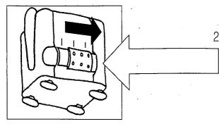
2. On the pump, locate the flow control lever on the pump's side.Set the flow-rate to maximum by moving the adjustment slider to the right-most (toward "+") position.
