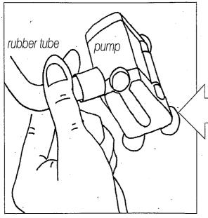
3. Attach the pump outlet to the rubber tube underneath the sculpture top.
