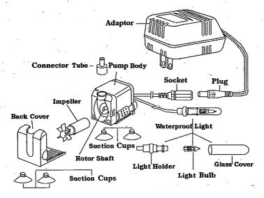
This product is an electrical submersible pump with a water-resistant lamp. When used with the supplied 12V AC-transformer adapter, this product may be used safely in the manner described in this manual. Take care to ensure that the lamp always remains submerged when in use at the risk of product damage or personal injury.
