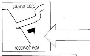
5. Run the excess pump cord out through the groove at the top of the rear wall of the reservoir.
