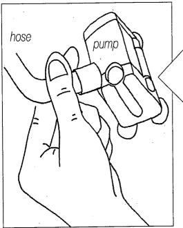
6. Holding the top half of the sculpture over the reservoir bottom, insert the rubber tube into the pump outlet. Tip: Insert your flattened hand in the space between the sculpture top and reservoir. Using two fingers to grasp the bottom of the hose, guide the hose into the pump outlet. Adjust the position of the pump as needed.
