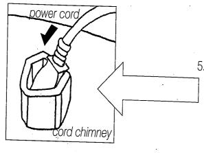
Locate the plug end of the pump cord and insert it through the cord chimney of the reservoir base, being sure to orient the plug in the proper direction that will allow it to fit through the cord chimney.
