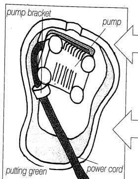
3. Measure about 2 1/2" of slack on the pump cord from the pump housing. With the underside of the pump facing you and the pump outlet oriented toward the fountain hole on the putting green, tuck the cord at the 2 1/2" mark under the cord bracket located on the underside of the putting green.
