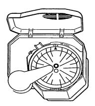
Turn Water Nozzle back into position, so that it sits over the Filter Holder.
