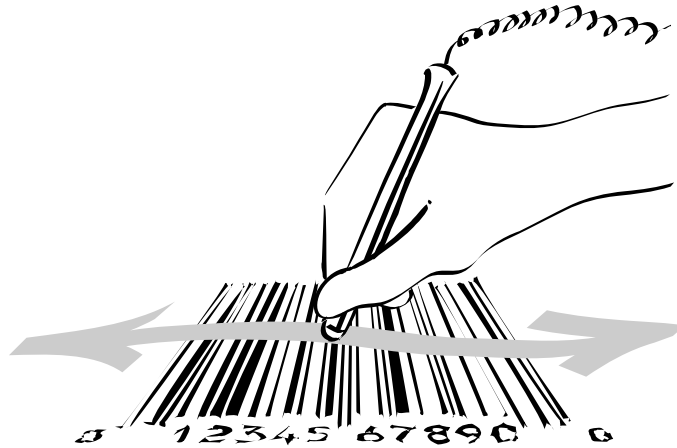
FIGURE 3. Scan the entire from barcode beginning outside the left edge
