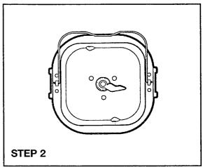
Position the Kneading Paddle on the Drive Shaft as shown.
