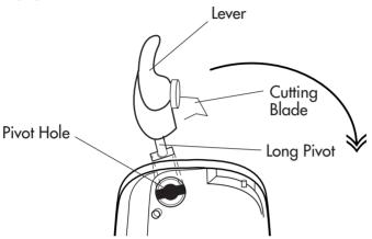
Unplug unit from electrical outlet. To remove lever, hold Can Opener facing you. Lift the lever upward and gently pull toward you.
