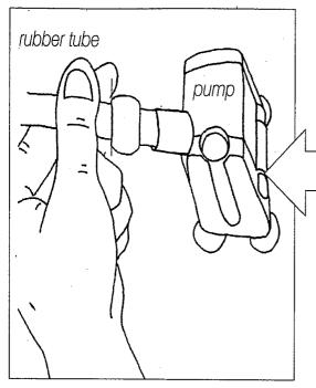
3. Insert the rubber tube of the Seashell panel through the hole of the rear panel. Attach the pump to the hose, making sure that the rear panel stays in place. The pump cord should face toward the center of the Seashell panel.
