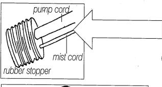
cord; the smaller hole is for the mist-maker cord. Leave enough cord slack for both the pump and mist-maker to permit convenient set up.
