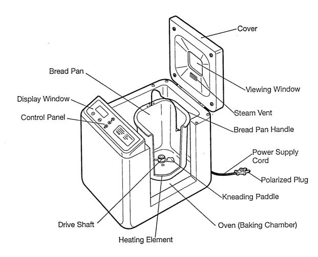
**Polarized Plug:** This appliance has a polarized plug (one blade is wider than the other). To reduce the risk of electric shock, this plug is intended to fit into a polarized outlet only one way. If the plug does not fit fully in the outlet, reverse the plug. If it still does not fit, contact a qualified electrician. Do not attempt to modify the plug in any way.
