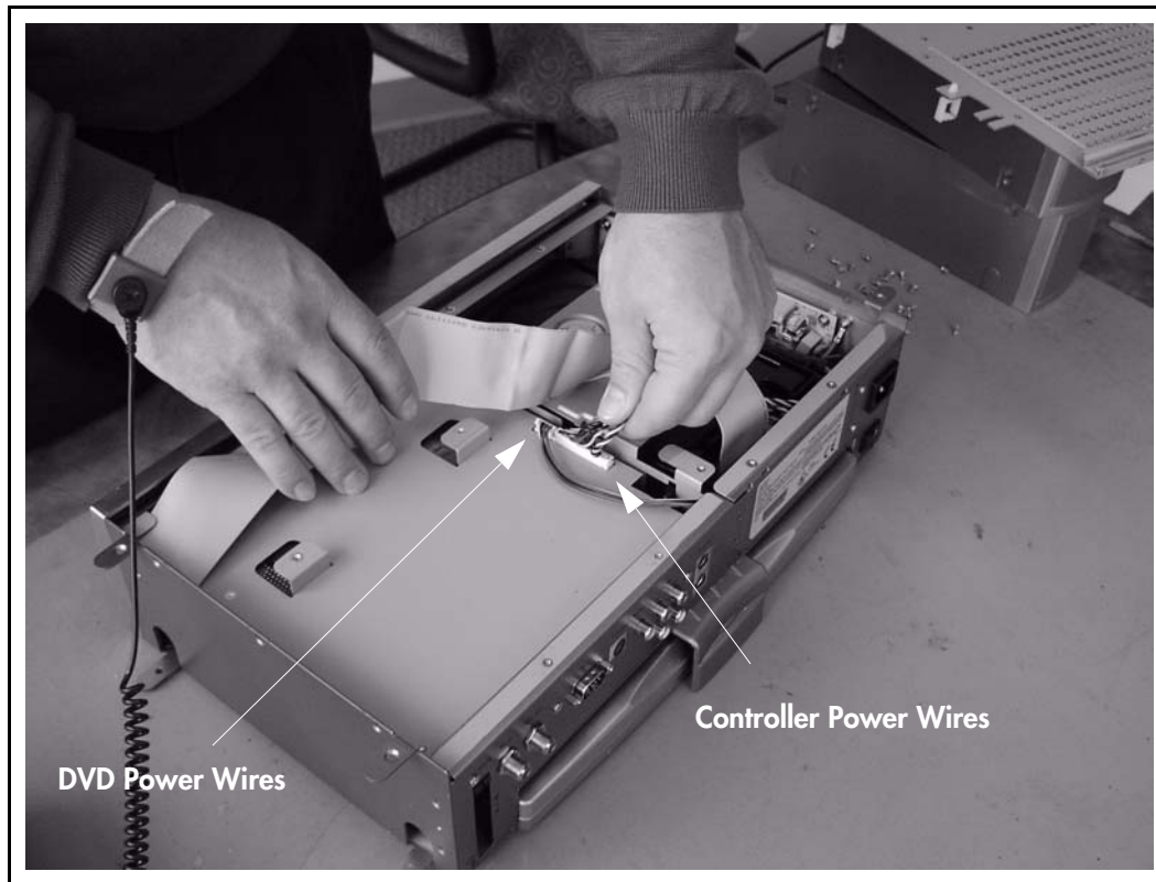
FIGURE 8. Removing the main controller (step 1)
