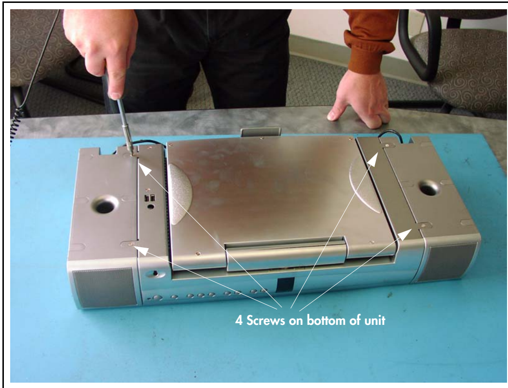
FIGURE 3. Removing the speakers (bottom view)
