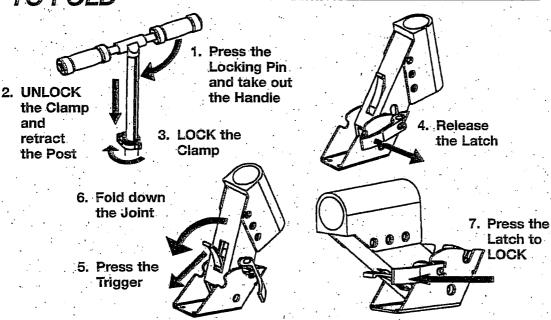
When locked correctly the Handlebar and Steering Height Pole should not change position.
