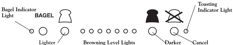
The Toasting Controls are located at the front of the Toaster. When the Toaster is plugged in, the Browning Level Lights will illuminate.
