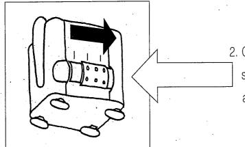
On the pump, locate the flow control leveron the pump's side. Set the flow-rate to maximum by moving the adjustment slider to the right-most (toward "+") position.
