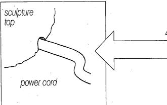
4. Lead excess pump cord through the cord groove at the back of the sculpture top.
